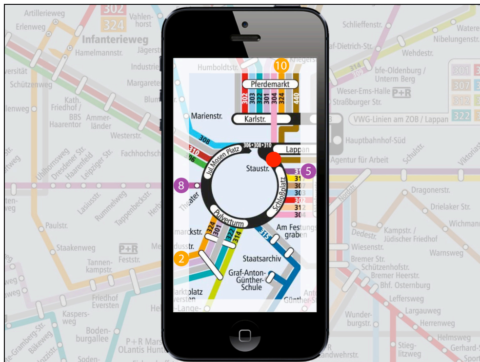
Figure 3. Sketch of a mobile application visualising a schematic public transportation network. The fringe displays the expected arrival of the next buses to come for two selected routes. The background shows parts of the off-screen network. (Gollenstede A, 2014; map: http://www.vwg.de )
