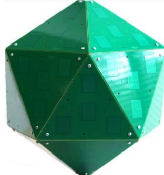
2011: 3rd proto, 80-element 3-dimensional – 35 cm diam.
